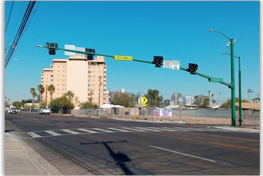
The Hawk Signal at 7th Avenue and Cocopah Street was Activated in December
